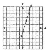
Place a point on the y-axis at -1. Slope is 3 or 3/1, so travel up 3 on the y-axis and over 1 to the right.
